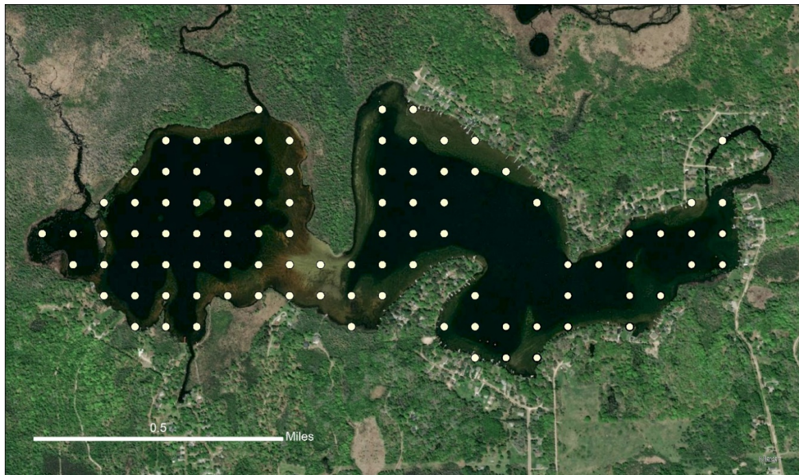
Figure 1. AuSable Lake littoral zone point-intercept sampling point locations (103 points established using GIS, 93 points surveyed).
